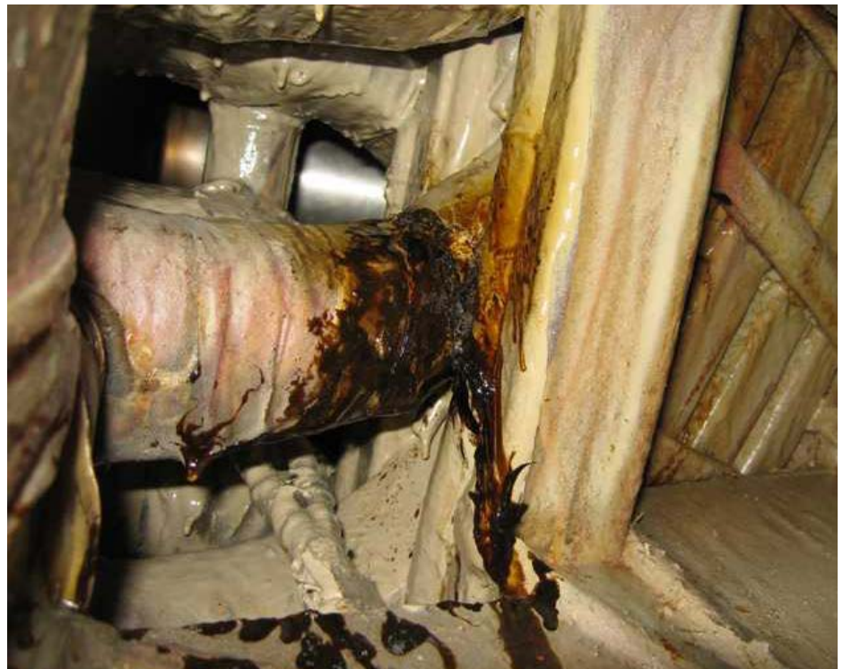
As-found generator stator bar insulation damage
